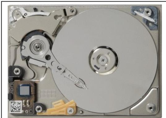
Exhibit 39: A modern disk storage device, manufactured by Seagate Technology
