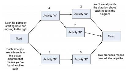
Figure 11.2 Step 1 Network Diagram
