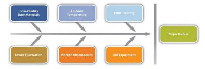
Figure 14.5 Cause-and-Effect (Fishbone) Diagram Source: http://pm4id.org/10/4/
