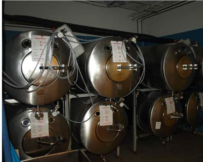
**Figure 7.15** Fermentation of grape juice into wine produces CO<sub>2</sub> as a byproduct. Fermentation tanks have valves so that the pressure inside the tanks created by the carbon dioxide produced can be released.
