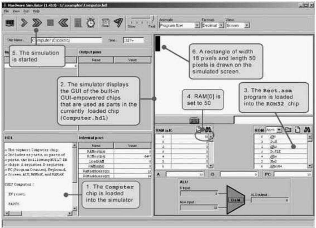
**Figure 5.11** Testing the Computer chip on the hardware simulator. The Rect program draws a rectangle of width 16 pixels and length RAM[0] at the top left of the screen. Note that the program is correct. Thus, if it does not work properly, it means that the computer platform on which it runs (Computer.hdl and/or some of its lower-level parts) is buggy.
