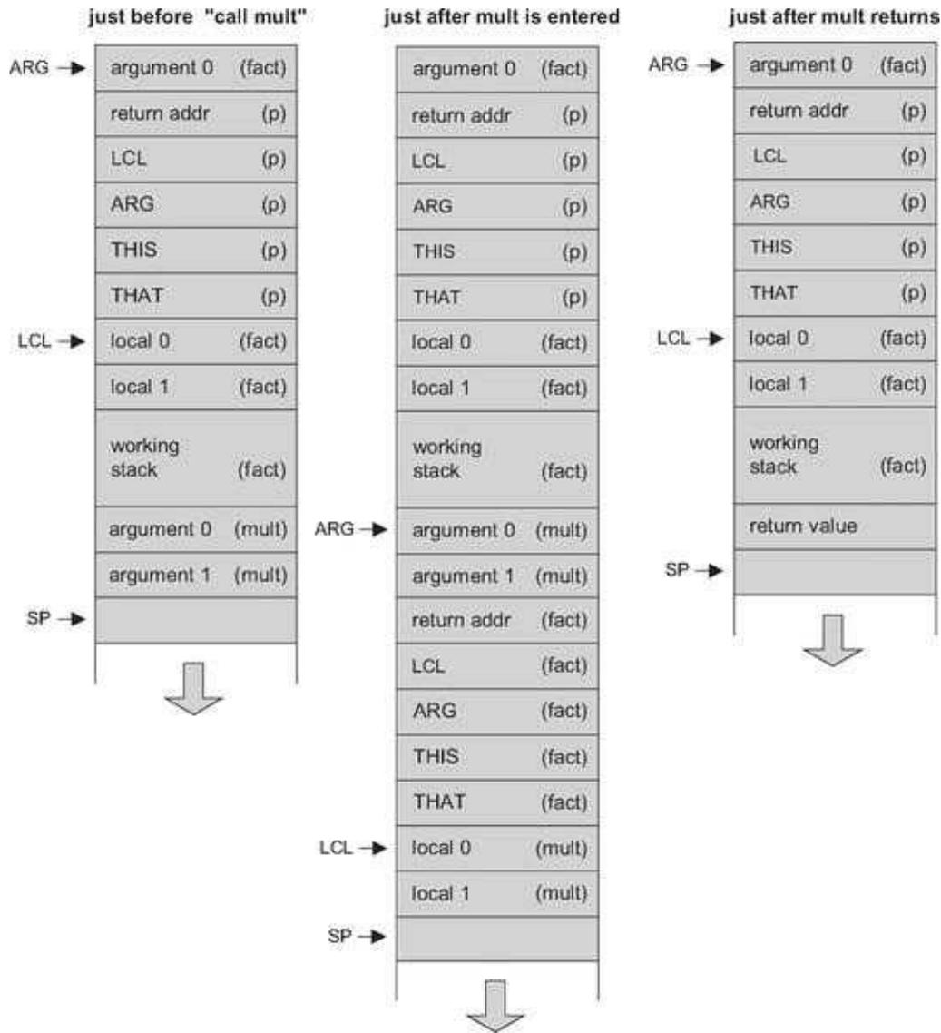
**Figure 8.8** Global stack dynamics corresponding to figure 8.7, focusing on the call mult event. The pointers SP, ARG, and LCL are not part of the VM abstraction and are used by the VM implementation to map the stack on the host RAM.
