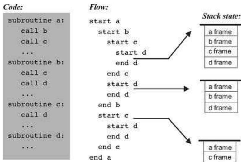
**Figure 8.3** Subroutine calls and stack states associated with three representative points in the program's life cycle. All the layers in the stack are waiting for the current layer to complete its execution, at which point the stack becomes shorter and execution resumes at the level just below the current layer. (Following convention, the stack is drawn as if it grows downward.)
