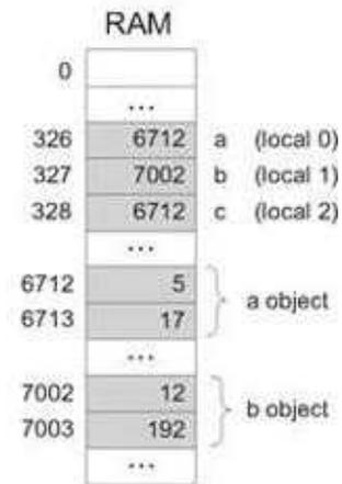
**Figure 11.3** Objects handling. Since memory allocations are run-time dependent, all the shown addresses are arbitrary examples.
