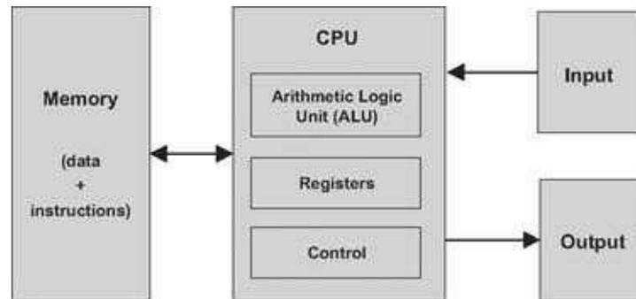
**Figure 5.1** The von Neumann architecture (conceptual). At this level of detail, this model describes the architecture of almost all digital computers. The program that operates the computer resides in its memory, in accordance with the “stored program” concept.
