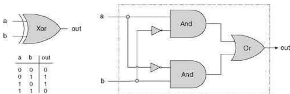
**Figure 1.5** Xor gate, along with a possible implementation.
