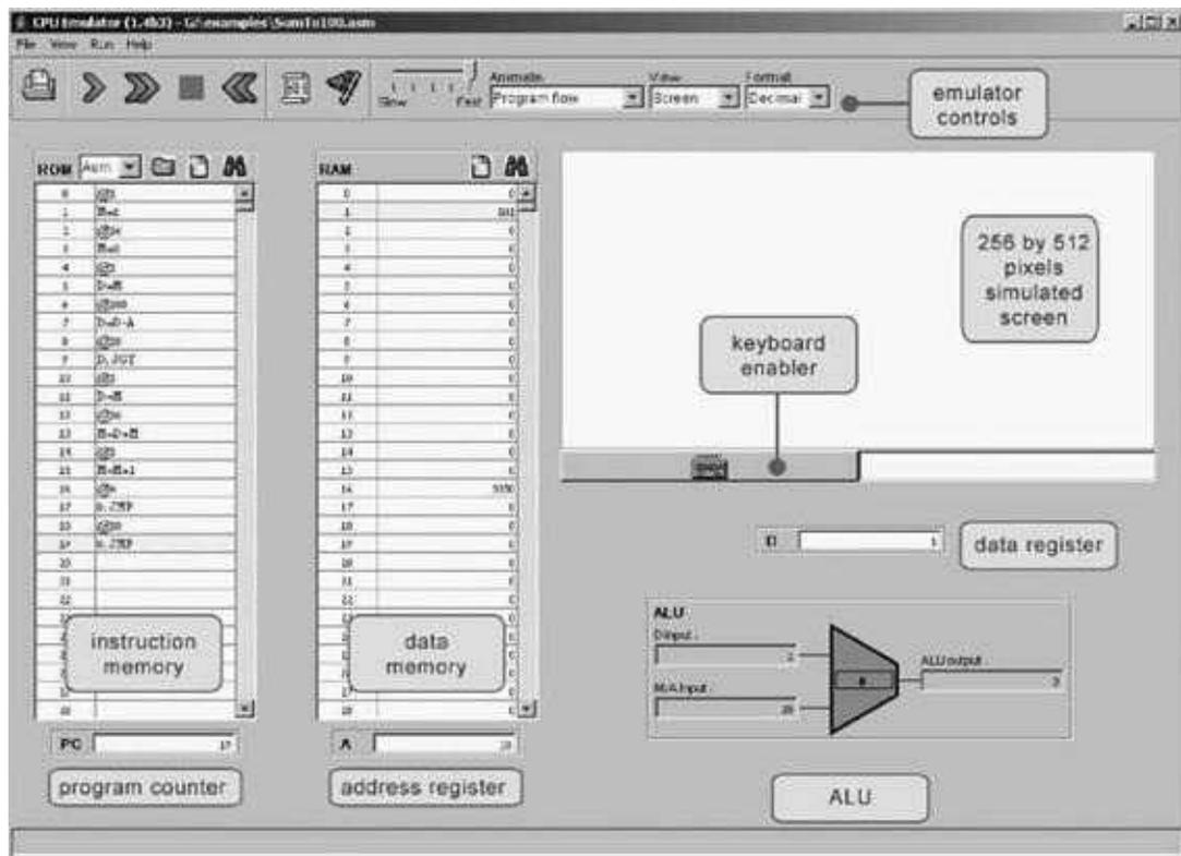
**Figure 4.8** The CPU emulator supplied with the book. The loaded program can be displayed either in symbolic notation (as shown in this screen shot) or in binary code. The screen and the keyboard are not used by this particular program.
