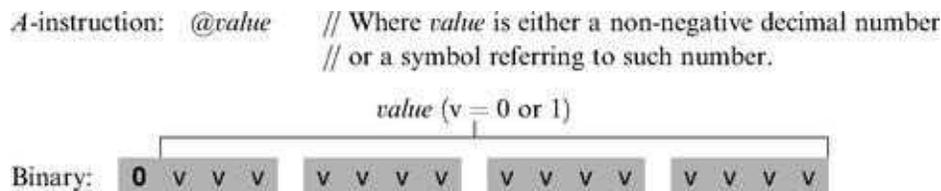
This instruction causes the computer to store the specified value in the A register. For example, the instruction `@ 5`, which is equivalent to `0000000000000101`, causes the computer to store the binary representation of 5 in the A register.
