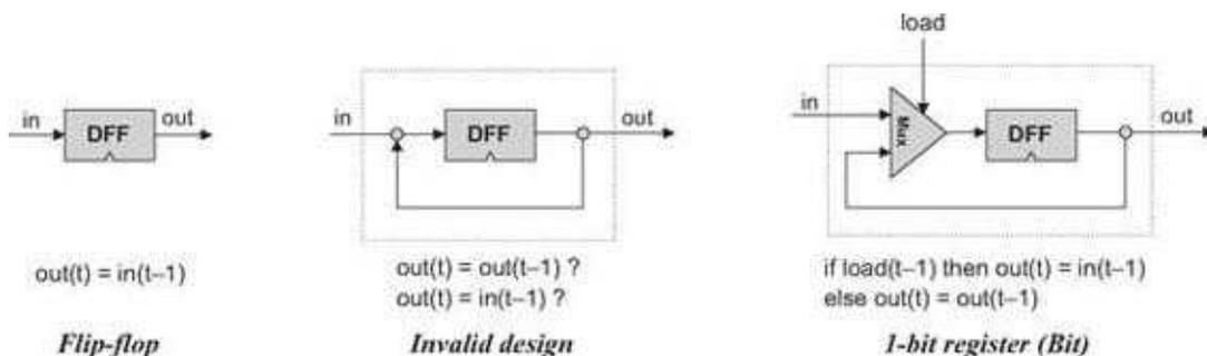
**Figure 3.1** From a DFF to a single-bit register. The small triangle represents the clock input. This icon is used to state that the marked chip, as well as the overall chip that encapsulates it, is time-dependent.
