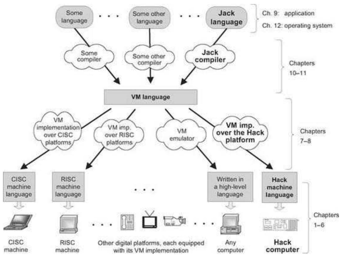
**Figure 7.1** The virtual machine paradigm. Once a high-level program is compiled into VM code, the program can run on any hardware platform equipped with a suitable VM implementation. In this chapter we start building the *VM implementation on the Hack platform* and use a VM emulator like the one depicted on the right.
