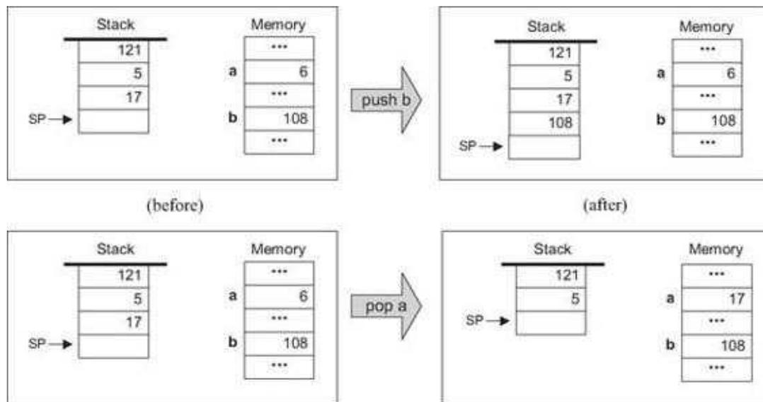
**Figure 7.2** Stack processing example, illustrating the two elementary operations *push* and *pop*. Following convention, the stack is drawn upside down, as if it grows downward. The location just after the top position is always referred to by a special pointer called *sp*, or *stack pointer*. The labels *a* and *b* refer to
