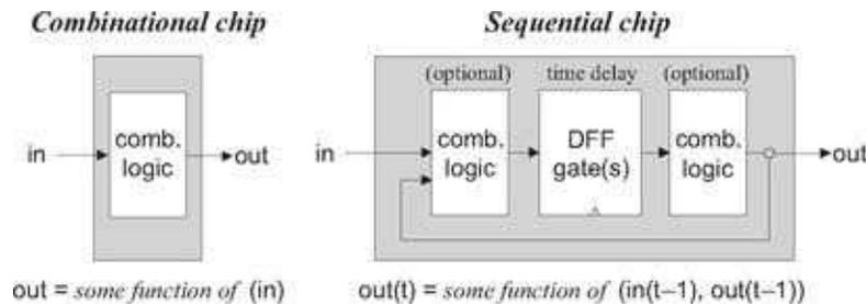
**Figure 3.4** Combinational versus sequential logic (in and out stand for one or more input and output variables). Sequential chips always consist of a layer of DFFs sandwiched between optional combinational logic layers.
