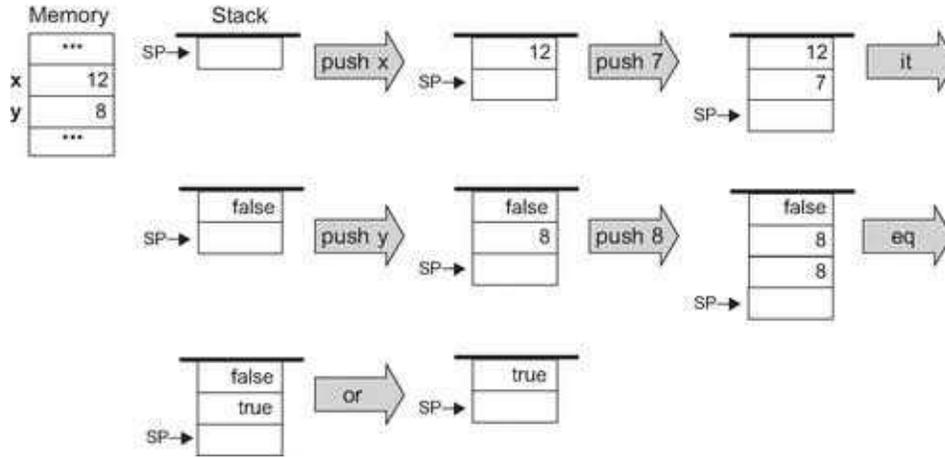
**Figure 7.4** Stack-based evaluation of logical expressions. This example evaluates the Boolean expression  $(x < 7) \text{ or } (y = 8)$ , assuming the initial memory state  $x = 12, y = 8$ .
