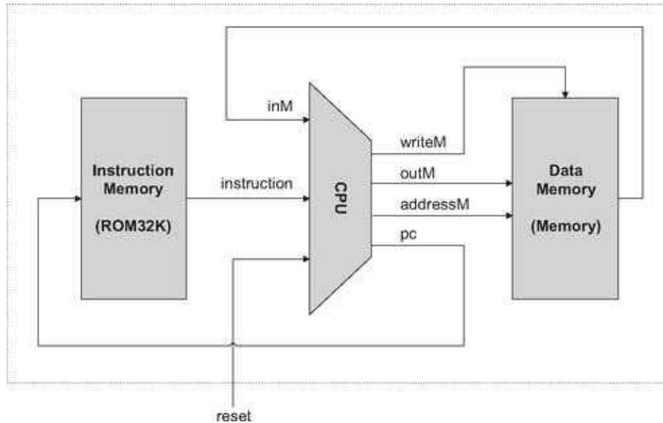
**Figure 5.10** Proposed implementation of the topmost Computer chip.
