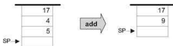
The stack version of other operations (subtract, multiply, etc.) are precisely the same. For example, consider the expression  $d=(2-x)*(y+5)$ , taken from some high-level program. The stack-based evaluation of this expression is shown in figure 7.3.
