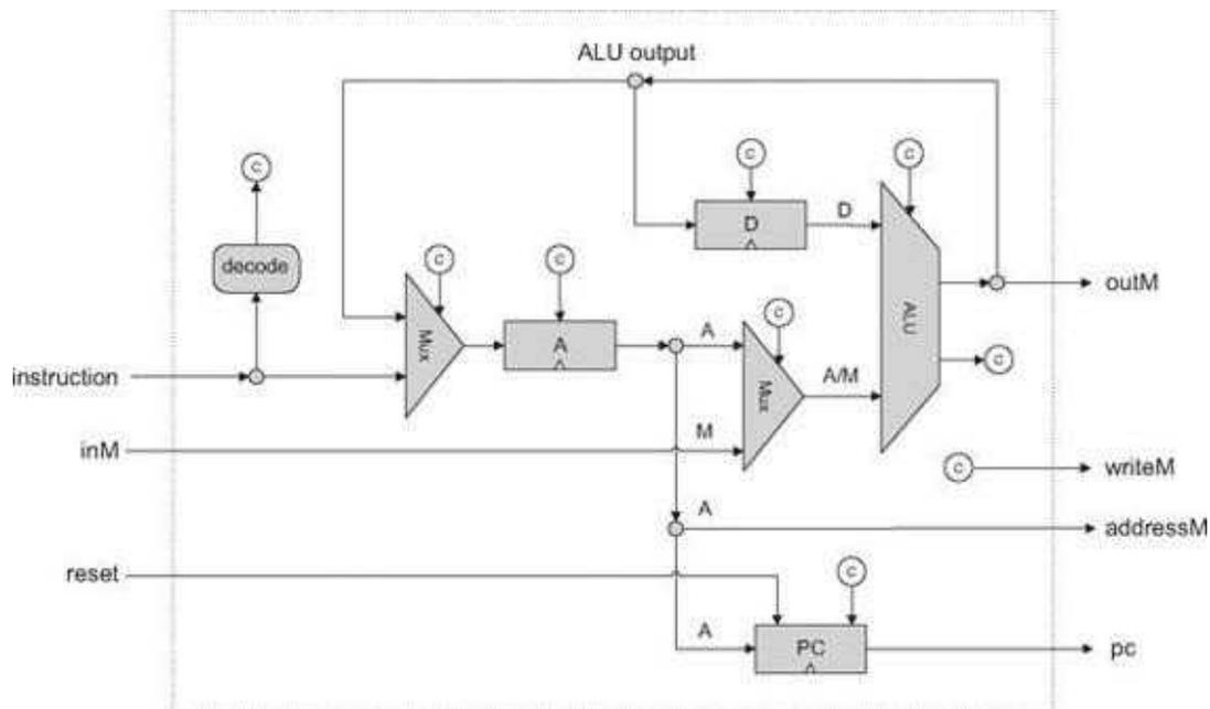
**Figure 5.9** Proposed CPU implementation. The diagram shows only *data* and *address paths*, namely, wires that carry data and addresses from one place to another. The diagram does not show the CPU's *control logic*, except for inputs and outputs of control bits, labeled with a circled “c”. Thus it should be viewed as an incomplete chip diagram.
