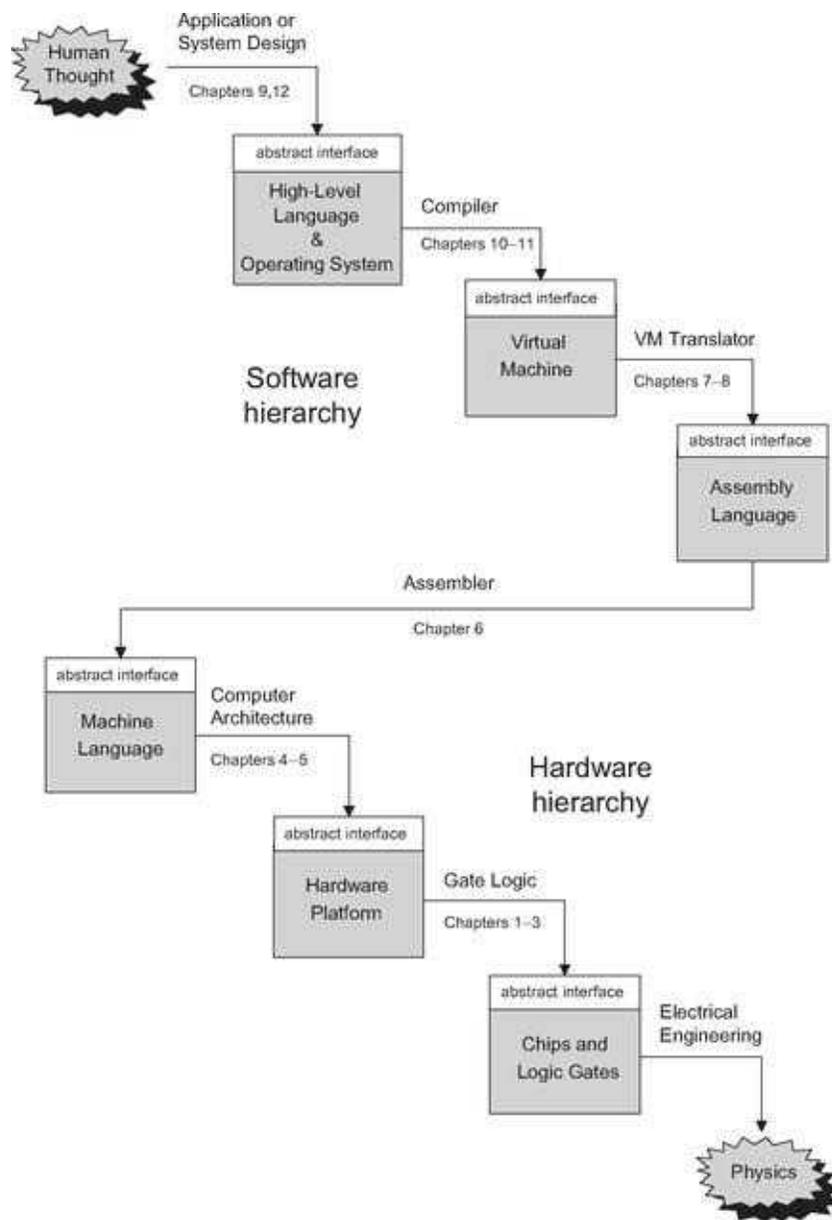
**Figure I.1** The major abstractions underlying the design of a typical computing system. The implementation of each level is accomplished using abstract services and building blocks from the level below.
