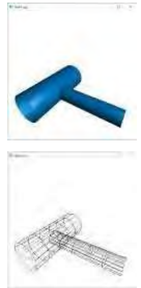
Figure 10.83: A T-pipe simulated by sticking one GLU cylinder into another.
