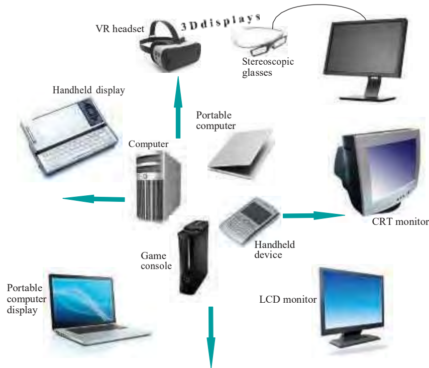
Figure 1.14: Output devices clockwise from the rightmost (surrounding processing devices in the middle): CRT monitor, LCD monitor, notebook, mobile phone, 3D displays including a VR headset and stereoscopic glasses tethered to a PC.
