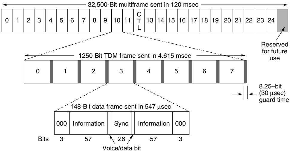
**Figure 2-48.** A portion of the GSM framing structure.
