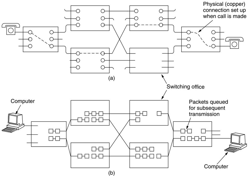
**Figure 2-42.** (a) Circuit switching. (b) Packet switching.
