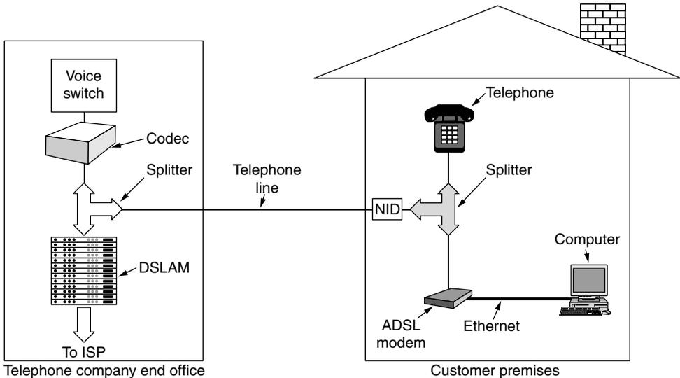
**Figure 2-35.** A typical ADSL equipment configuration.
