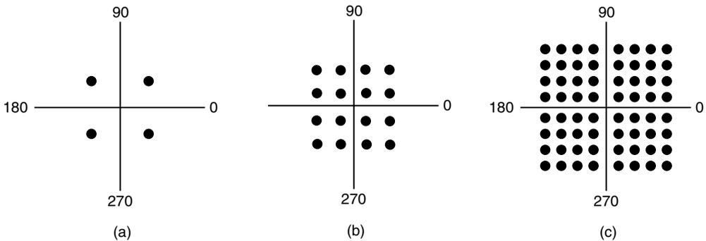
**Figure 2-23.** (a) QPSK. (b) QAM-16. (c) QAM-64.
