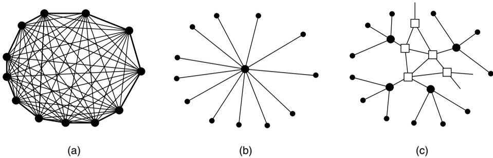
**Figure 2-29.** (a) Fully interconnected network. (b) Centralized switch.
