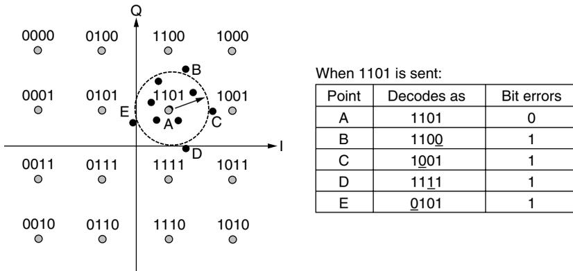
Figure 2-24. Gray-coded QAM-16.
