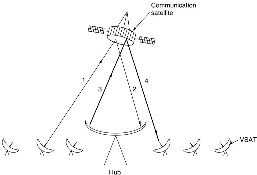
**Figure 2-17.** VSATs using a hub.
