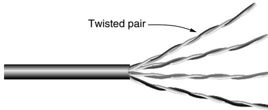
**Figure 2-3.** Category 5 UTP cable with four twisted pairs.
