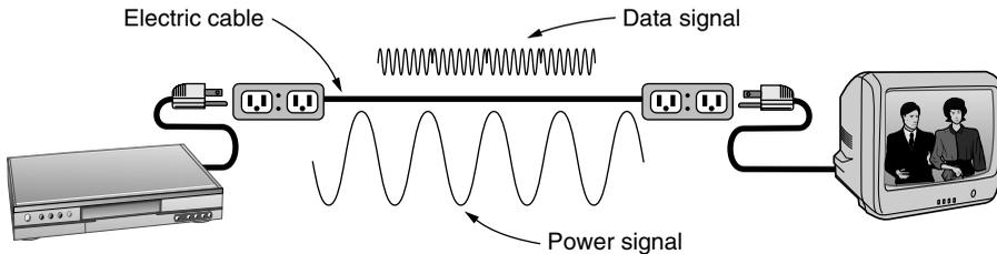
**Figure 2-5.** A network that uses household electrical wiring.
