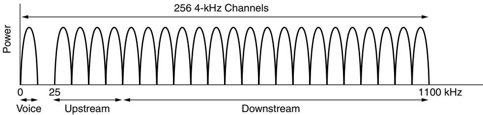
**Figure 2-34.** Operation of ADSL using discrete multitone modulation.
