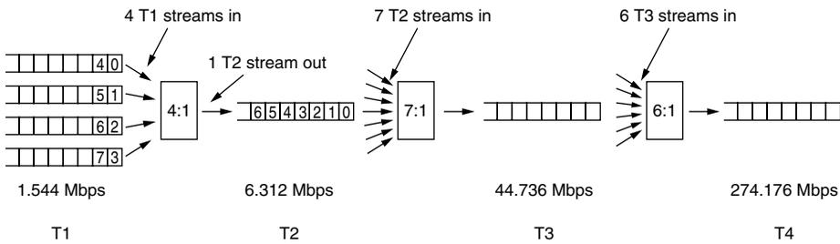
Figure 2-38. Multiplexing T1 streams into higher carriers.
