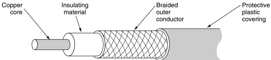
**Figure 2-4.** A coaxial cable.
