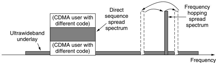
**Figure 2-11.** Spread spectrum and ultra-wideband (UWB) communication.
