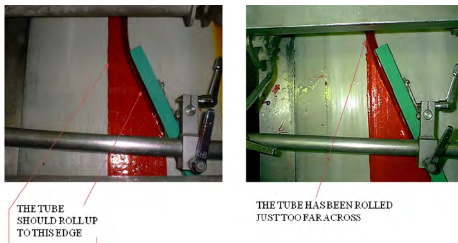
Figure 19.8. Incorrect plough set-up
